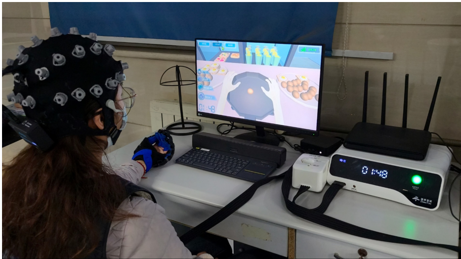
Figure 2. Photograph of the KI-BCI training system. The system comprises an EEG acquisition module for real-time signal recording, a computing unit that analyzes neural data and delivers real-time visual and auditory cues, and an integrated feedback mechanism that provides triggered tactile and motor assistance during task performance.
